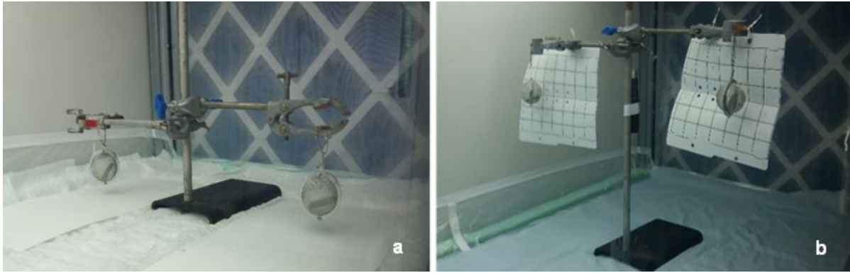
Fig. 4. Set up of wind tunnel experiments: (a) variation 1 - white sticky traps beneath tea infusers (upwind); (b) variation 3 - sticky traps behind tea infusers (upwind)
