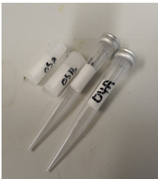
Fig. 3. Controlled release pheromone dispensers: polyethylene vials (left) and pipette tips (right)
